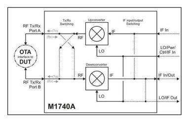
Figure 2. M1740A block diagram
